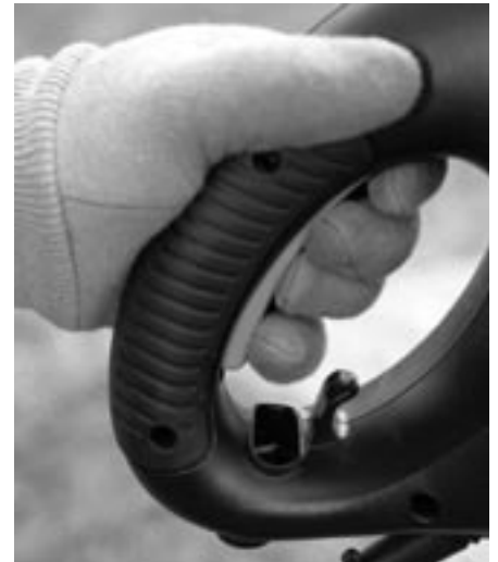
Figure 3-7: Squeezing rear trigger switch to start trimmer
